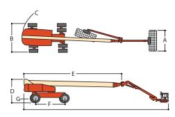
**Standard Features** Platform: 36 x 96 in. (0.91 x 2.44 m) Side Entry 8 ft (2.44 m) JibPLUS° Boom Selectable Capacity Envelope 180° Hydraulic Platform Rotator AC Receptacle in the Platform 5 Degree Tilt Alarm/Indicator Light All Motion Alarm Swing-Out Engine Tray 12V DC Auxiliary Power Hourmeter Control ADE® System Full-time 4WD 3 Selectable Steering Modes Drive-out Extendible Axles Oscillating Axle **Proportional Controls Gull-Wing Hoods** 445/50D710 Foam Filled Rim Protector Lug Tread Tires
